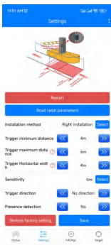
Figure 7: Select installation method
